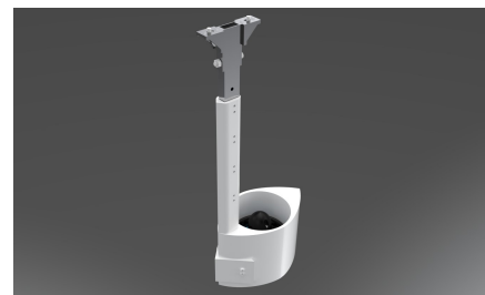
Fig. 3. Heave thruster design
